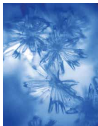
Drug crystals located on top of a biodegradable film. The film is used to build an active implant.
